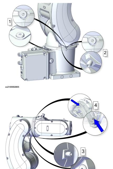
Axis 4 of IRB 1010 is calibrated with an internal fixed calibration pin and a fixed calibration block. It does not use the calibration tools for Axis Calibration method.
